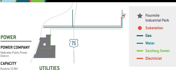
Existing 12.5kV distribution circuit has 5MW of available capacity
